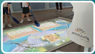
ActiveFloor Mobile Max consists of a mobile installation box with a projector, a computer and a motion-detecting camera that turns the (vinyl)floor projection into a touch-screen that can detect multiple objects.
